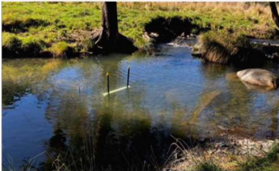
Figure 3 Time integrated suspended sediment sampler installed at site.
